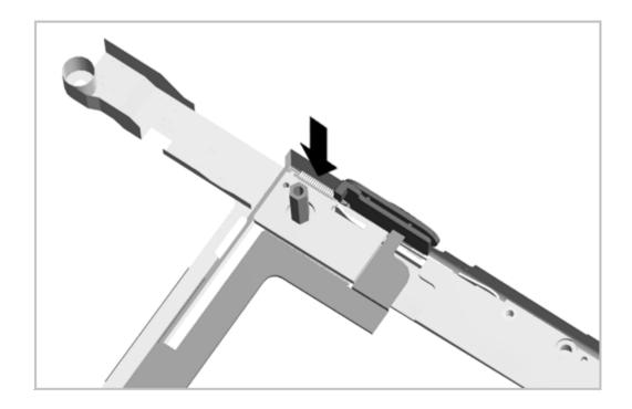
Figure 5-46. Installing the MultiBay Release Assembly
